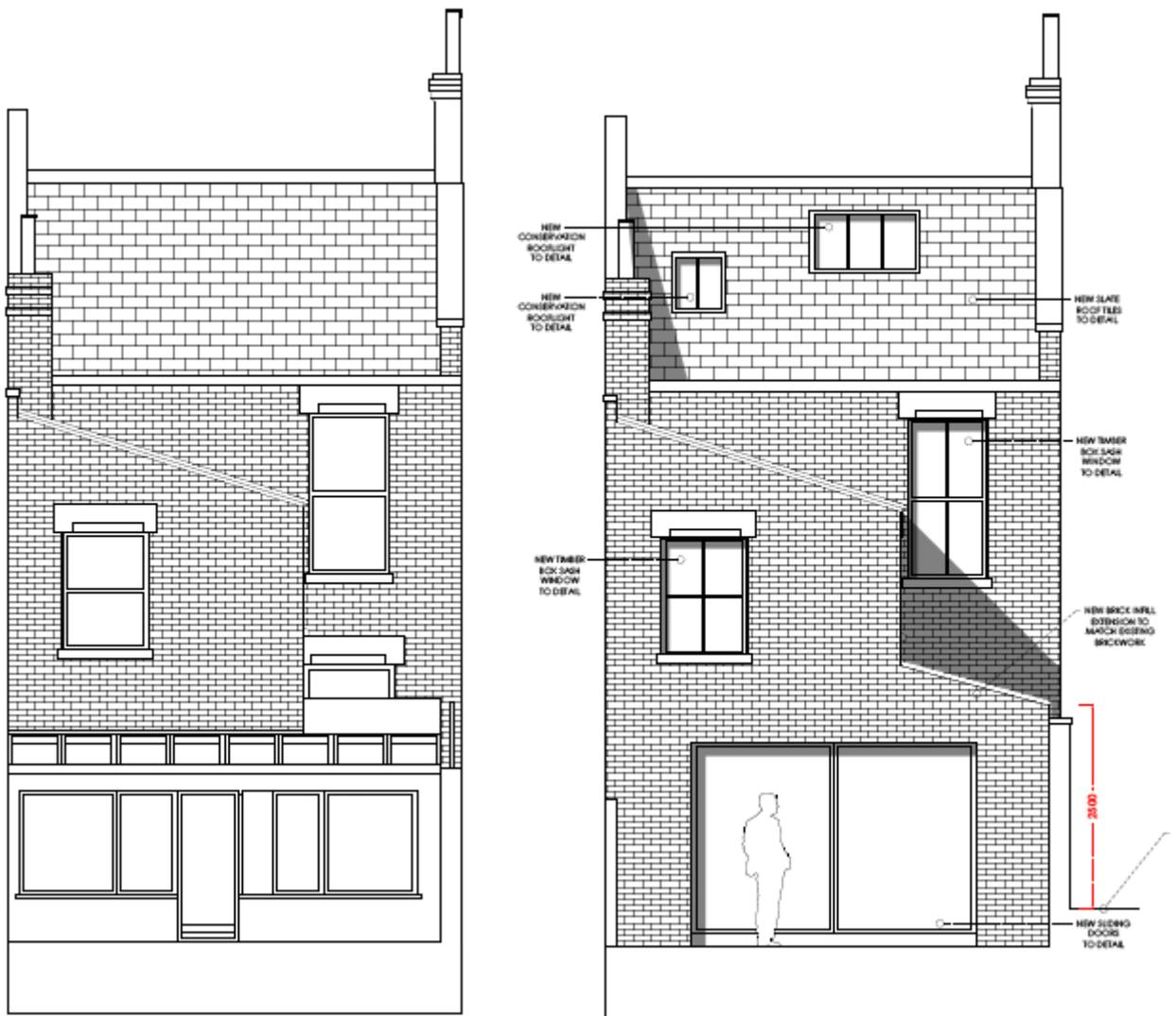
Figure 2: existing (left) and proposed (right) rear elevation
