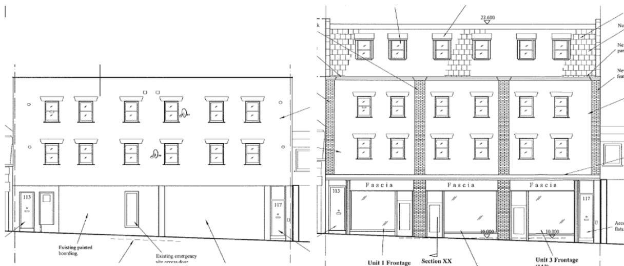
**Figure 2 Existing and proposed front elevations**
