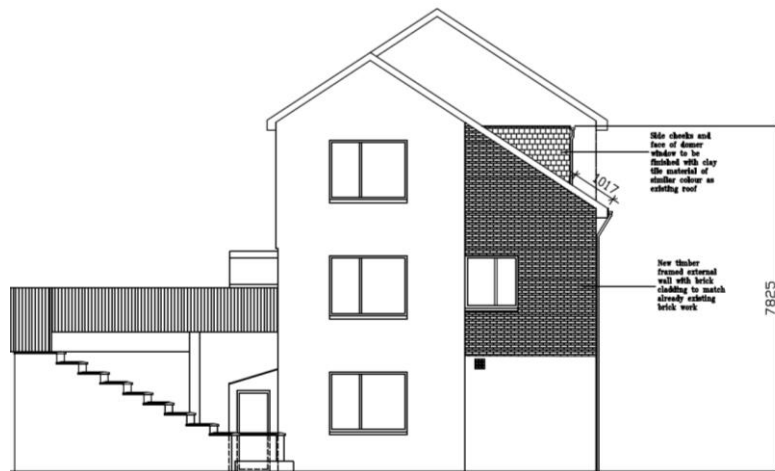
Figure 2 Proposed Side Elevation
