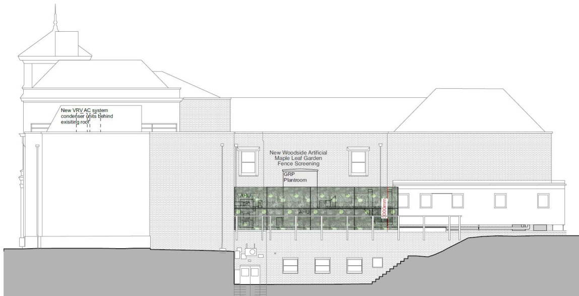
Proposed West Elevation With Plant Screening
