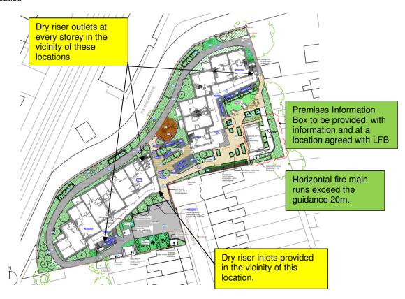
This does involve horizontal runs in excess of the guidance 20m, yet the hydraulic design of the system should be straightforward to ensure that the performance of the fire main is satisfactory. It is noted that a dry main can serve storeys up to 50m, and as our top storey is only approximately 10m above access level and it is more difficult to pump vertically (against gravity and the friction of the pipe) than horizontally (no gravity forces)
