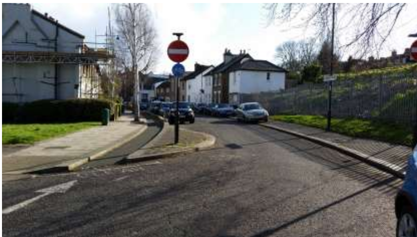
One-way street with contraflow cycling facility on Stanstead Road near Forest Hill.
